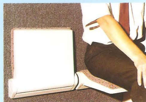
To increase seating capacity tip-up seats are provided in all vestibules on the train except those on the catering vehicle.
