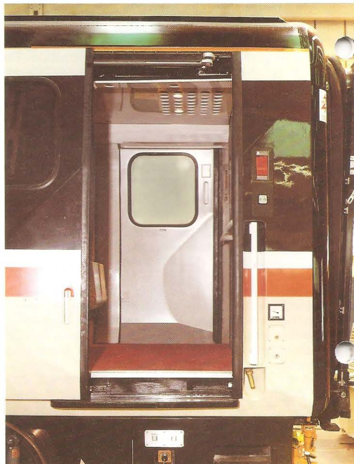
The operating mechanism for the sliding-plug door can be seen on this view.
